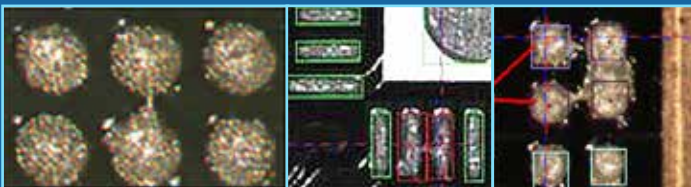
Low Solder Bridge Inspection
