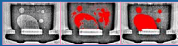
Void Defect Gray-level Based AI Algorithm
