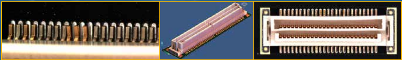
Lifted Lead on Connectors
